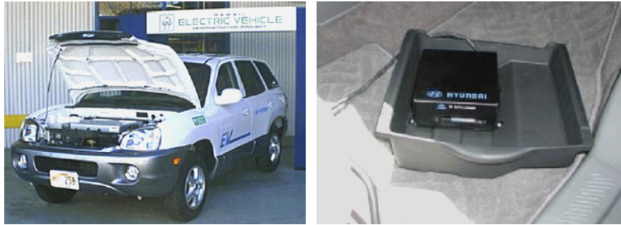
Fig. 2. Hyundai Motor Company's Santa Fe e-SUV and the on-board data logger used for data acquisition.
